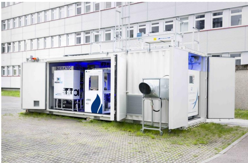
The world's first integrated Power-to-Liquid (PtL) test facility to synthesize fuels from the air-captured carbon dioxide. (Photo: P2X project/Patrick Langer, KIT)
